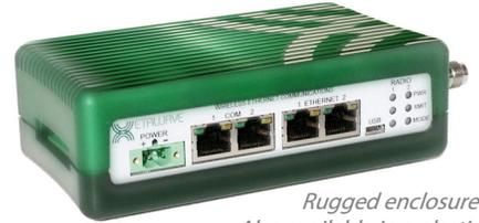
*Rugged enclosure. Also available in a plastic enclosure and as a board level product.*
